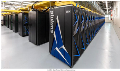
256 cabinets, 18 nodes per cabinet => 4608 nodes
